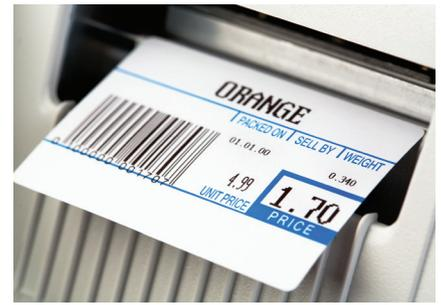
Direct thermal printing requires a heat sensitive label material. Due to direct contact between the print head elements and the heat sensitive material, the exposed heat from the print head elements cause a colour change in the material to create the printed image. For thermal transfer printing, a thermal transfer ribbon is additionally required to print the ink onto any sort of substrate.
